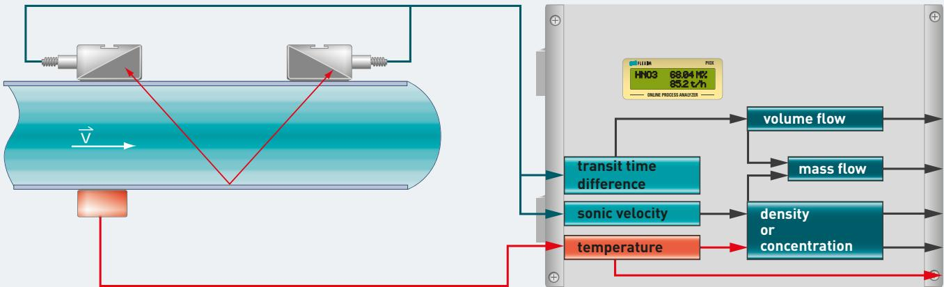
Two ultrasonic transducers are mounted to the pipe wall, and are alternately sending and receiving ultrasonic signals. Measuring the difference in the transit time between the two signals, the flow velocity ( $v$ ) and the volume flow, based on the pipes inner diameter, are accurately calculated.
